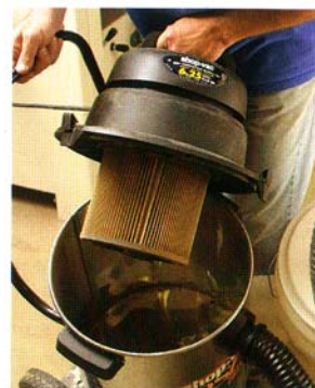
Clean filter means full power. With the Dust Deputy attached, the filter stays surprisingly clean.
