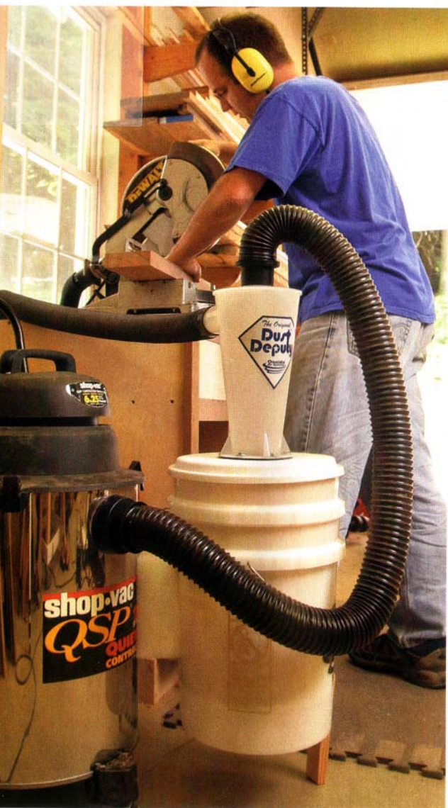
Joined at the hip. The Dust Deputy can be bolted to the canister of almost any shop vacuum.
